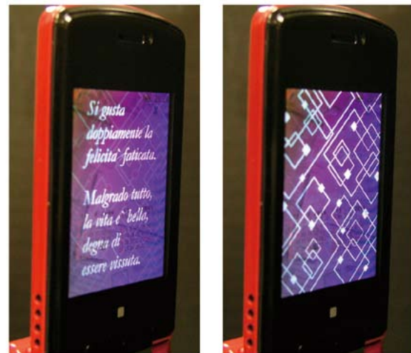
Fig. 9 Patterned masking images for production Veil View LCDs.
