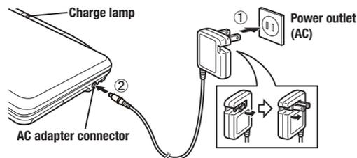
**2** When charging is complete, the charge lamp will turn off.
