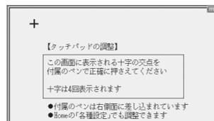
**5** Pull out the stylus and use it to accurately touch each center of the four "+" characters displayed on the touch pad on the display. Then do the same to the four "+" characters displayed on the handwriting pad (small screen).
